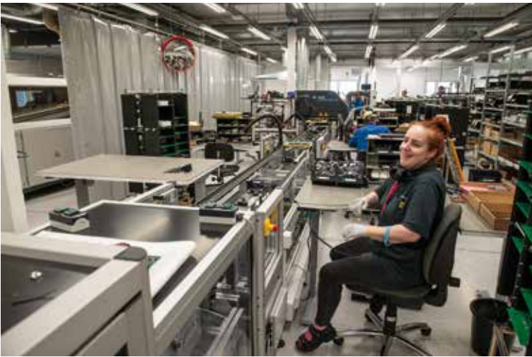
Satu Leiviskä performs visual inspection and manual placement. In the background is the new wave soldering machine, where the line sends the placed circuit boards.
