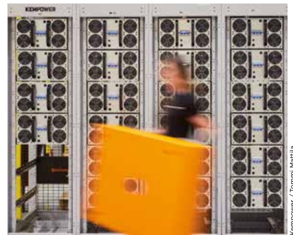
Power modules in production. The power unit can be equipped with one to four modules, each with a capacity of 50kW.
