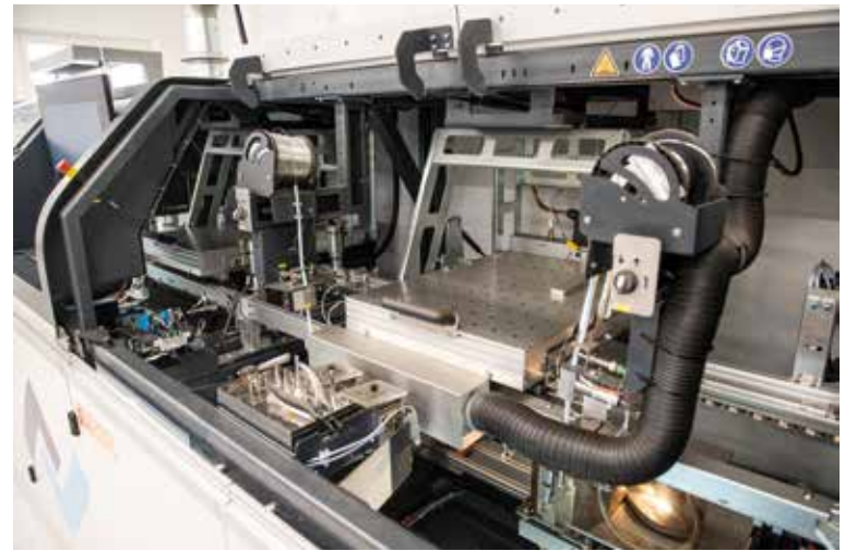
A look inside the selective soldering machine. During operation, the covers are closed and nitrogen gas prevents tin oxidation.
