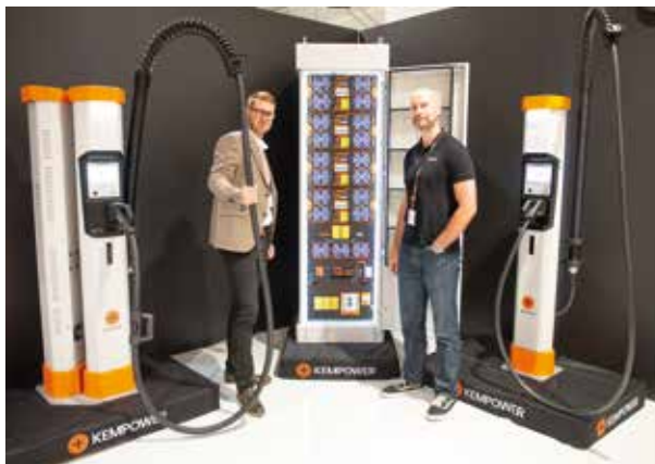
Petri Kettunen and Tuomas Laitila, with a liquid-cooled satellite on the left and a regular one on the right. In the middle is the power unit.
