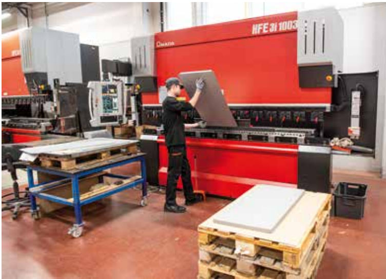
The new Amada HFE3i press brake completes the row of older press brakes and brings more speed and comfort to the work.
