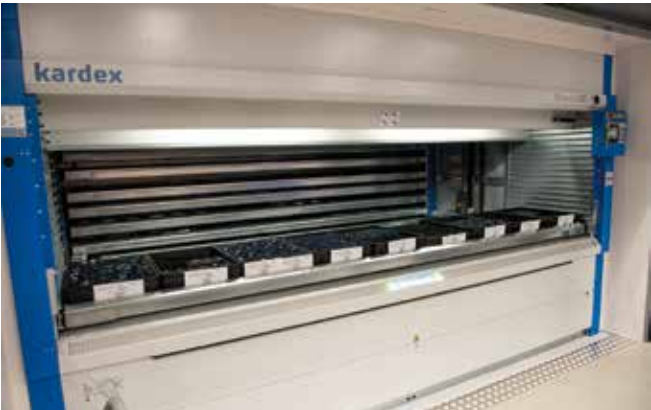
The new Vertical Lift Module, which works on the elevator principle, is four metres wide and seven metres high.
