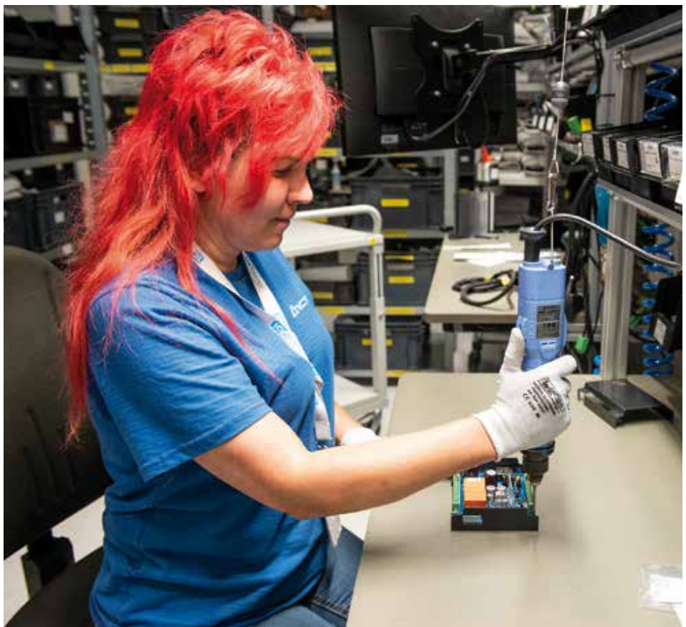
The final assembly of Arcteq products takes place at the company’s own factory. Here, Marjo Verkkomäki attaches the circuit board to the device’s case.
