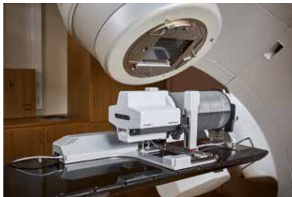
Delta4 Phantom+ is here equipped with the HexaMotion platform that simulates the patient’s breathing and movement and helps ensure the correct radiation dose to the target.
