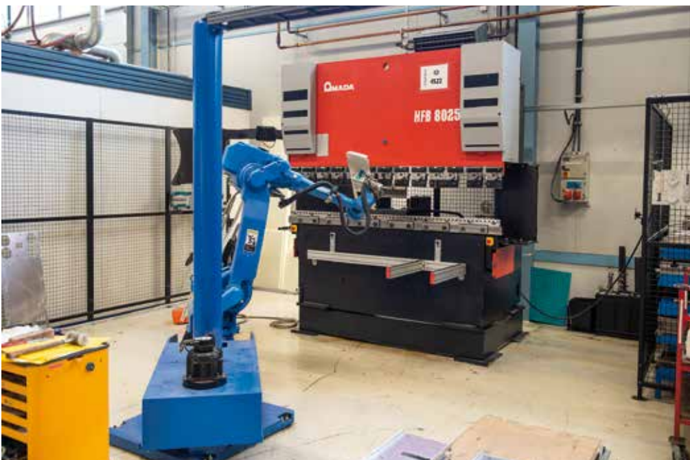
Amada press brake equipped with a Yaskawa arm robot has brought Klaukkala facility more capacity for the production of sheet metal parts.
