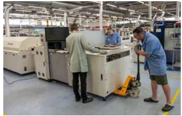
The reception unit is being placed after the AOI device.
