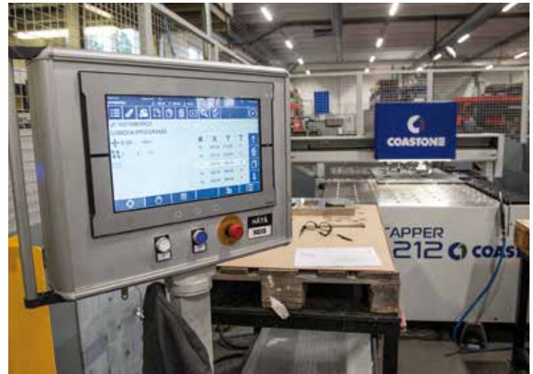
The handy touch screen of the TapOne Multitapper machine enables easy programming of threading and sinking. Alternatively, it is possible to import a finished CAM file to the machine.
