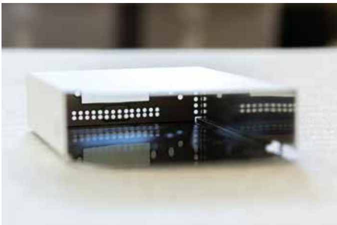
The enclosure painted in the jig has no paint at all inside.
