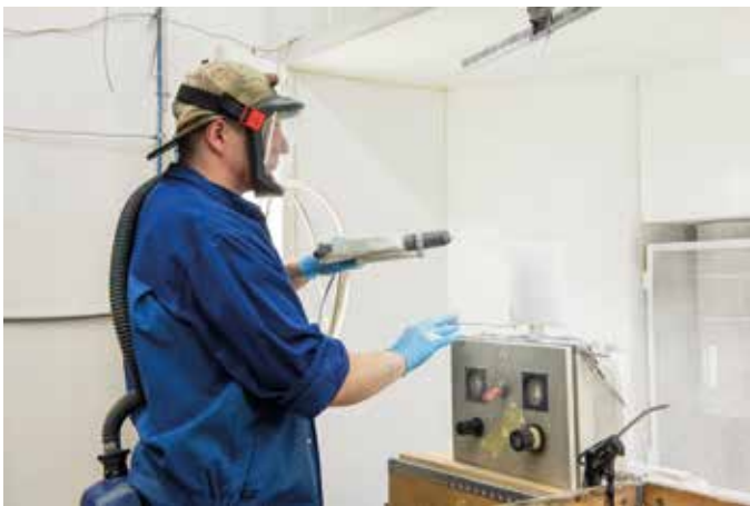
Painter Reido Pohla paints an enclosure in a painting jig.
