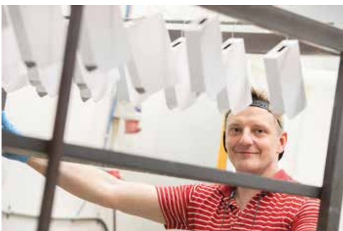
Reido Pohla fills the transport rack with painted enclosures going to the oven.
