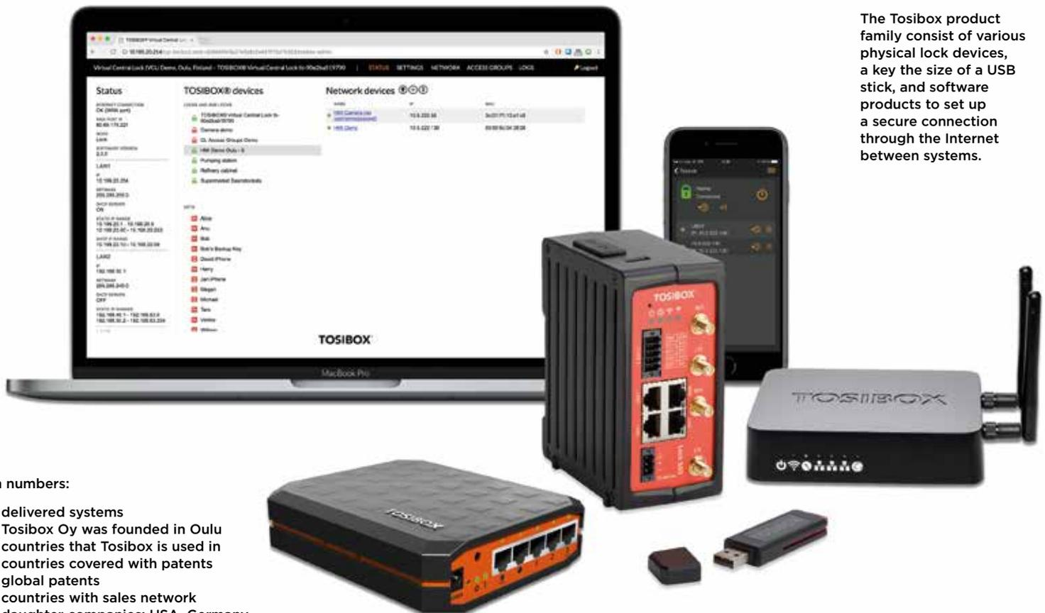
The Tosibox product family consist of various physical lock devices, a key the size of a USB stick, and software products to set up a secure connection through the Internet between systems.
