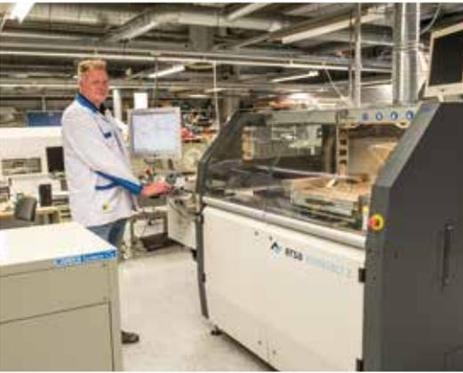
Elektroniikan 3K-tehdas has many pieces of equipment and services that Darekon can use. In the lefthand image Harri Reinikainen presents a selective soldering machine that is the latest acquisition at the plant. In the middle there is a handmade
