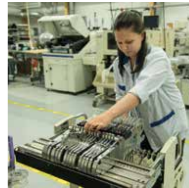
Emilia Jääskeläinen is preparing component cassettes for the placement machine for manufacturing the next product.
