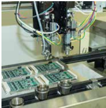
An automated coating robot spreads selective coating on desired parts of the circuit board.
