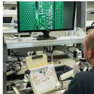
After reflow sharp eyes examine the flawlessness of placement and soldering.
