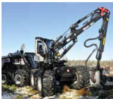
The Logset harvester gets over 70 per cent more power and 20-30 per cent lower fuel consumption with its Visedo diesel-electric drivetrain.
