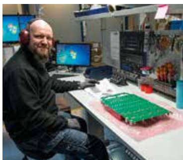
Visedo's PC-boards are large and heavy. The baseboards and copper are thick.
