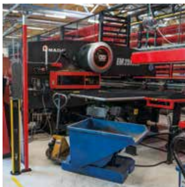
The new FMS system acquired for Darekon's Klaukkala facility three years ago is servo-operated, conserves an essential amount of energy and needs no hydraulic oil.
