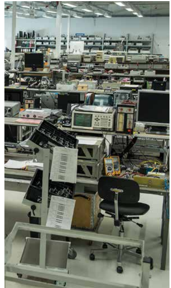
The functional testing of completed boards has its own area, equipped with all necessary test instruments.
